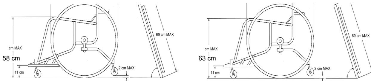
In all cases the height is measured from the floor to the highest point on the seat platform including the cushion if one is used.
